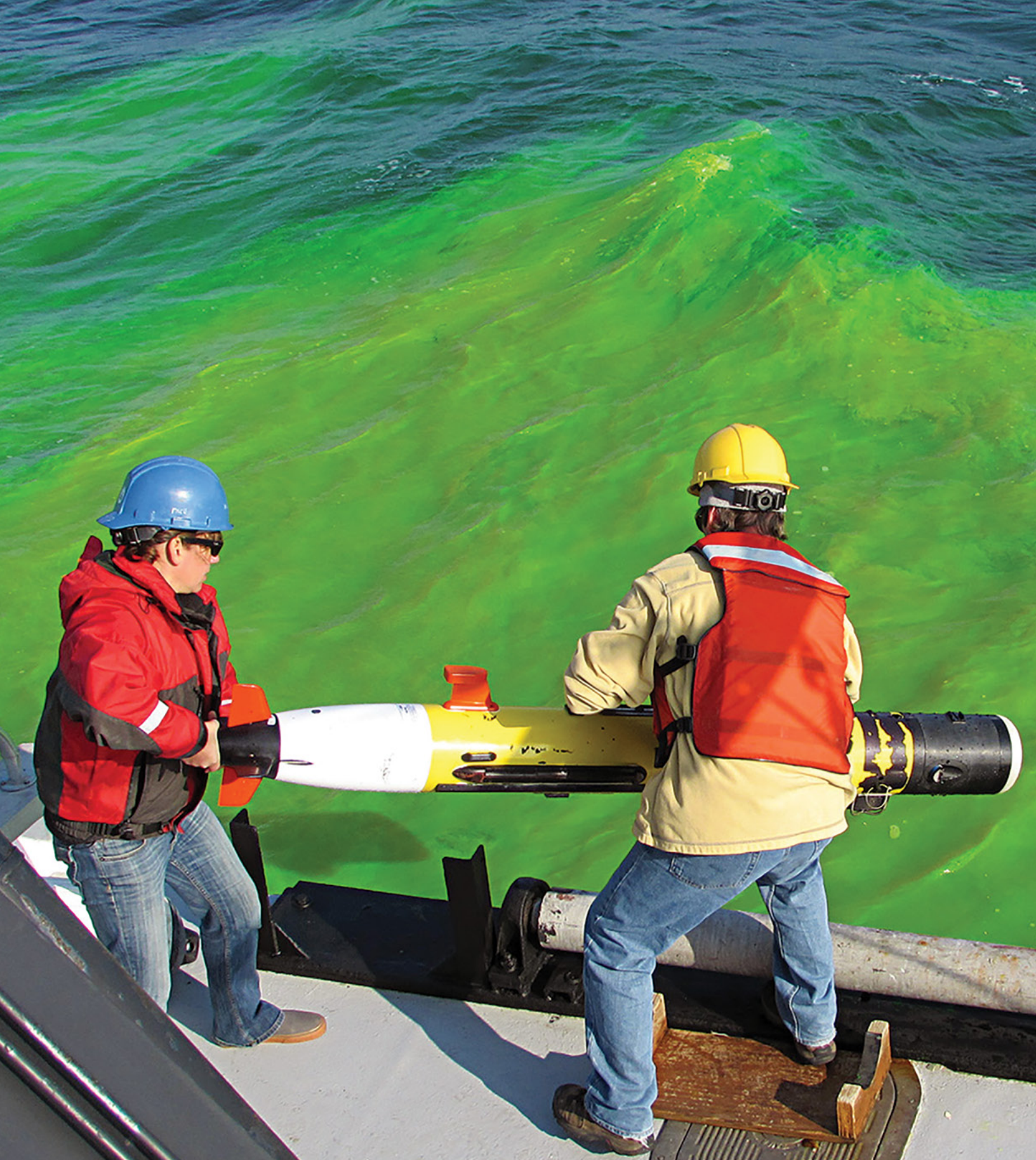
Staff from the Woods Hole Oceanographic Institution (WHOI) deploy a REMUS autonomous underwater submersible to test its ability to track oil spills. The REMUS was developed by WHOI's Oceanographic Systems Lab. (Photo by Erin Koenig, WHOI)
